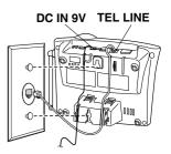
For a wall plate, plug the modular cord's other end into the wall plate jack, then align the base's keyhole slots with the wall plate studs and slide the base downward to secure it.
